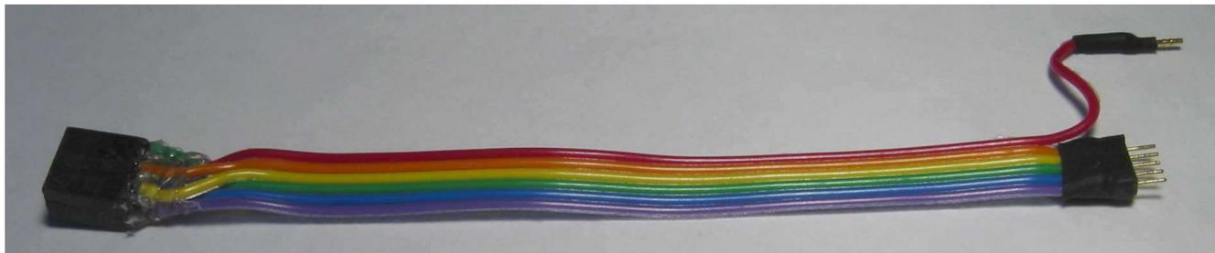
**Figure 5:** An example ISP adapter cable for MEGAbitty. A 6-pin 0.01” pitch socket (left) connects to the programmer. A 5-pin 0.05” pitch header (right) plugs into MEGAbitty’s ISP connector, and a free-floating wire connects to RESET.
